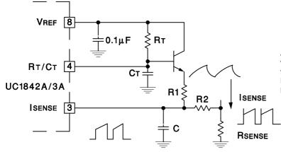
A fraction of the oscillator ramp can be resistively summed with the current sense signal to provide slope compensation for converters requiring duty cycles over 50%. Note that capacitor, C, forms a filter with R2 to suppress the leading edge switch spikes.
