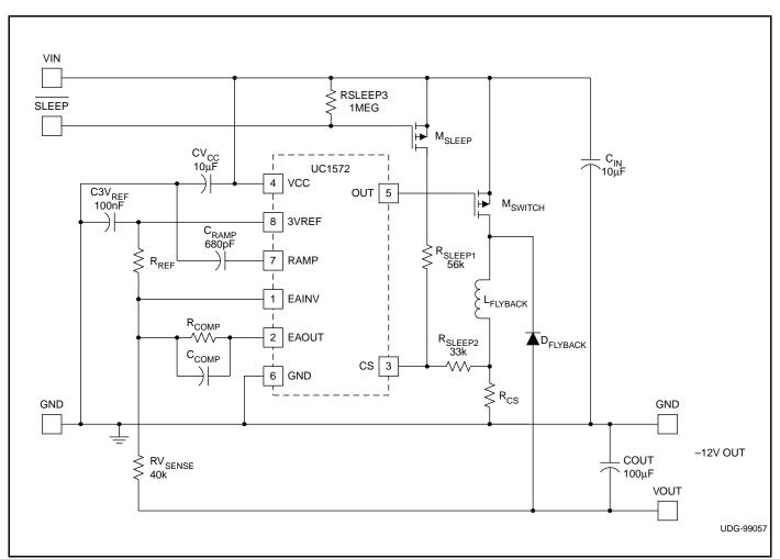
Figure 2. Typical application: +5V to -12V flyback converter.
