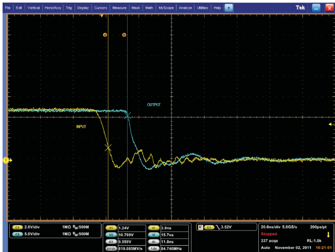
Figure 36. TurnOff Propagation Delay ( C_L = 1.8 \text{ nF} , V_{DD} = 12 \text{ V} )
