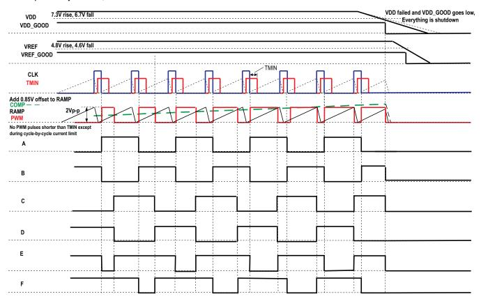
Figure 5. UCC28950-Q1 Timing Diagram
