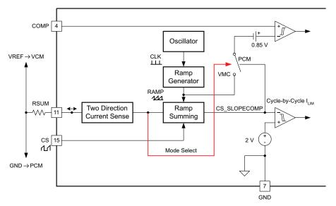
Figure 14 shows the operational logic of the slope-compensation circuit.
