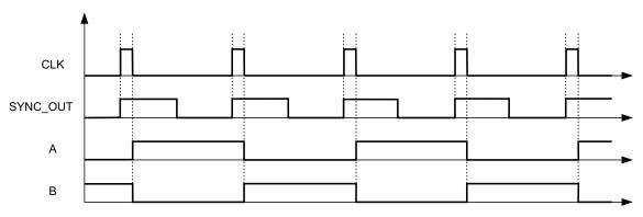
Figure 21. SYNC\_OUT (Master Mode) Timing Diagram
