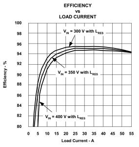
Figure 53. Efficiency of the Prototype Phase-Shifted Converter  $(V_{IN} = 300 \text{ V}, 350 \text{ V} \text{ and } 400 \text{ V}, V_{OUT} = 12 \text{ V})$
