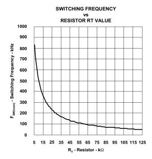
Figure 13. Converter Switching Frequency f<sub>SW(nom)</sub> Over Resistor RT Value
