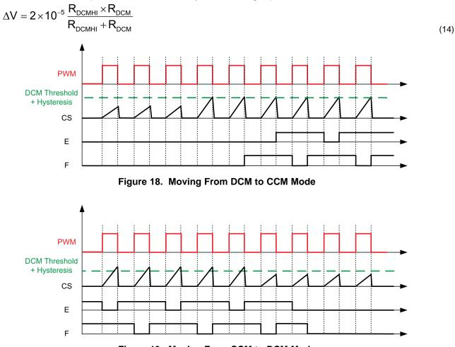
Figure 19. Moving From CCM to DCM Mode
