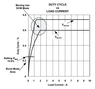
Figure 17. Duty-Cycle Change Over Load-Current Change
