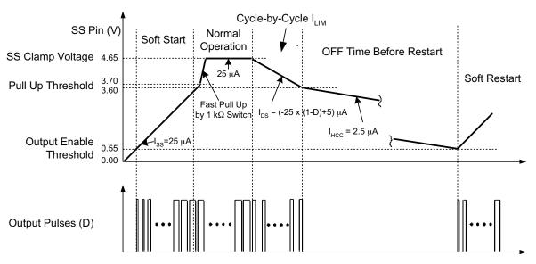
Figure 20. Timing Diagram of Soft-Start Voltage  $V_{SS}$
