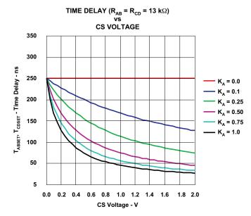
Figure 7. Delay-Time Set  $t_{ABSET}$  and  $t_{CDSET}$ (Over CS Voltage Variation and Selected K<sub>A</sub> for R<sub>AB</sub> and R<sub>CD</sub> Equal 13 kΩ)
