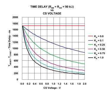
Figure 8. Delay-Time Set  $t_{ABSET}$  and  $t_{CDSET}$ (Over CS Voltage Variation and Selected K<sub>A</sub> for R<sub>AB</sub> and R<sub>CD</sub> Equal 90 k $\Omega$ )
