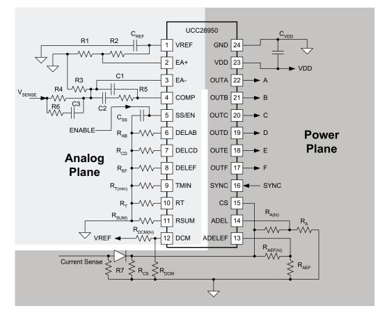
Figure 24. Layout Recommendation for Analog and Power Planes
