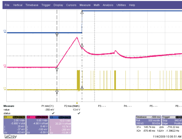
图 6. Start-Up Sequence Waveforms (Ch1 (Y), PFCDRV, Ch2 (R), V CC_A , Ch3 (B), DUT V O )
