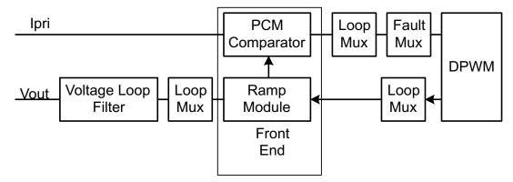
Figure 44. Peak Current Detection Function
