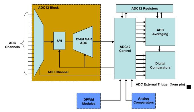
Figure 26. ADC12 Control Block Diagram
