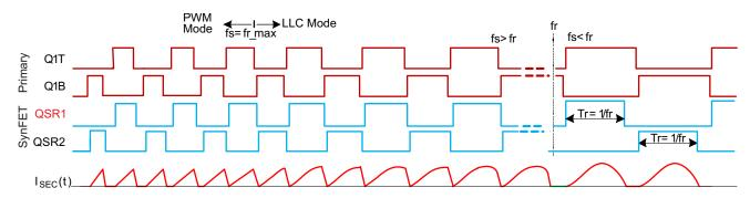
Figure 13. LLC Waveforms
