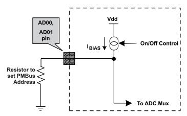
Figure 24. PMBUS Address Detection Method
