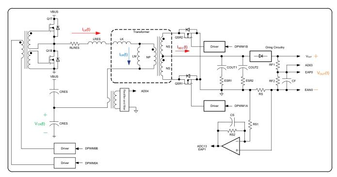
Figure 14. Secondary-Referenced Half-Bridge Resonant LLC Control With Synchronous Rectification
