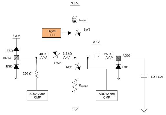
Figure 28. Simplified Current Sharing Circuitry
