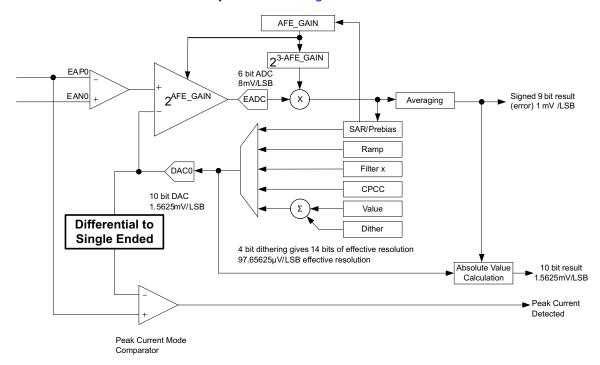
Figure 45. Differential to Single-Ended Comparator Function
