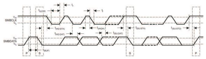
Figure 1. IC/SMBUS/PMBUS Timing Diagram<sup>2</sup>
