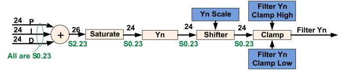
Figure 18. Output Section of the Filter
