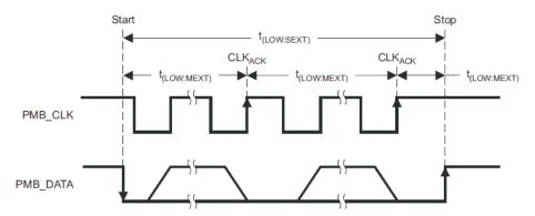
Figure 2. Bus Timing In Extended Mode
