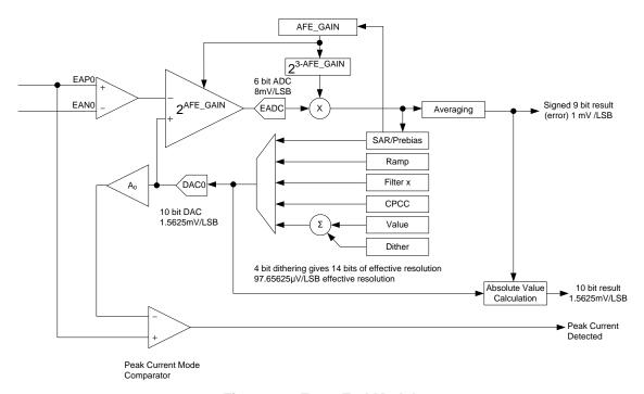
Figure 10. Front End Module
