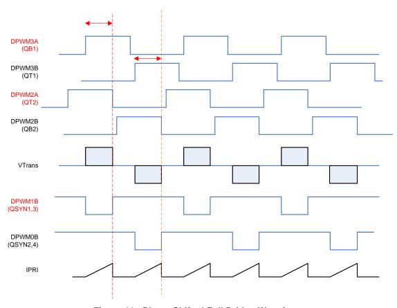
Figure 11. Phase-Shifted Full Bridge Waveforms
