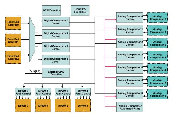
Figure 23. Fault Mux Block Diagram
