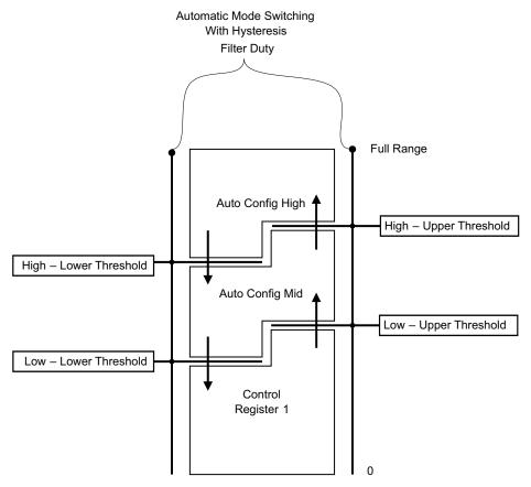
Figure 15. Automatic Mode Switching
