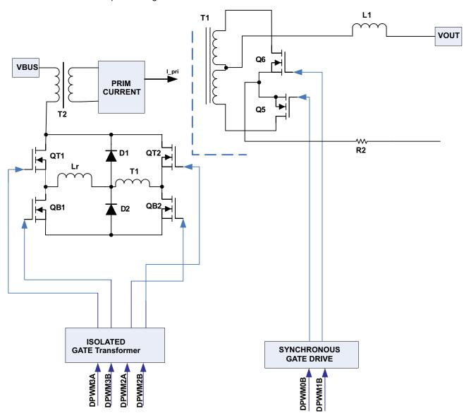
Figure 38. Schematic - PSFB Power Stage
