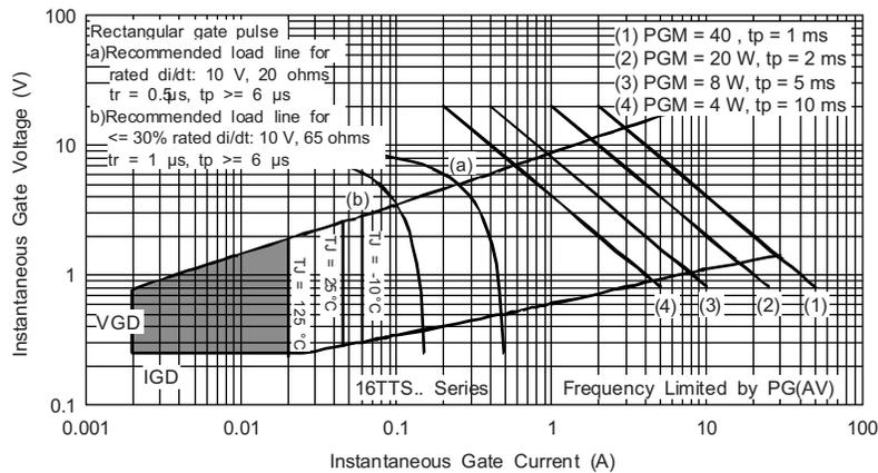
Fig. 9 - Gate Characteristics
